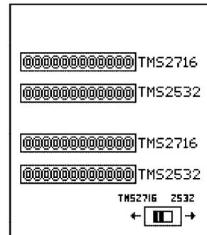
The illustrations below show the adapter base configured for the TMS2716 (left) and the TMS2532 (right). Note the position of the 24 pin socket and the slide switch for each device.
